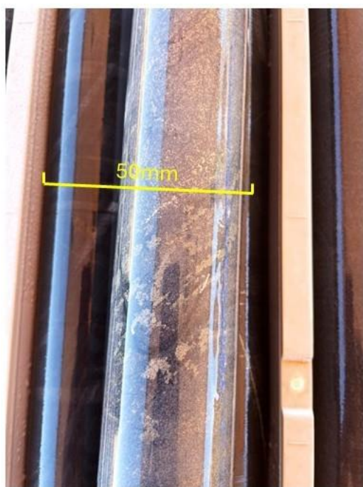
JUD001 - 520.4m example of chalcopyrite (copper) mineralisation
