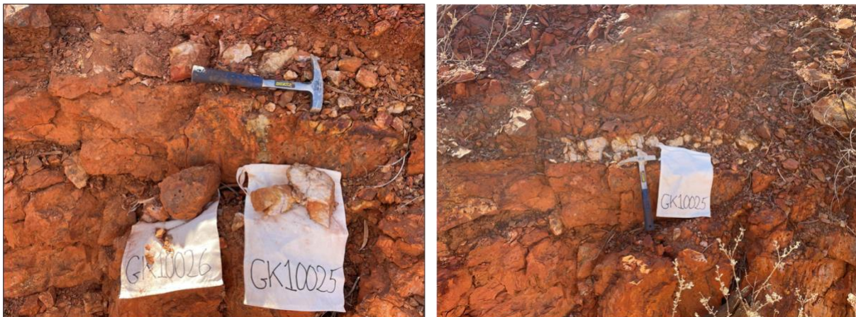
Figure 7 - Rock chip samples collected showing low angle quartz vein with pyrite alteration in wall rock.
