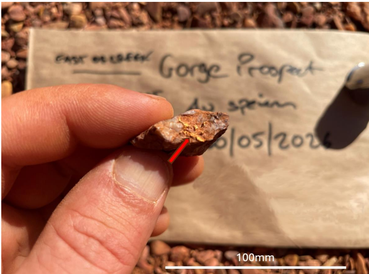
Figure 2 - Visible gold in a quartz vein sample understood to have been sourced from mullock heaps associated with the eastern shaft at the Gorge Mine. Coarse free gold is observed along fractures and veinlets within the quartz vein samples.
