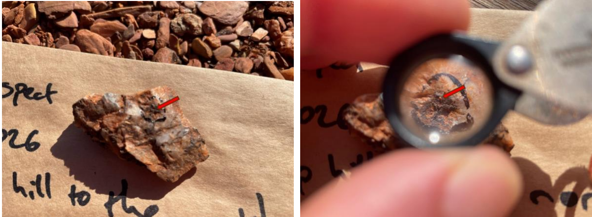
Figure 6 - Visible gold in altered quartz vein sample understood to have been sourced from a costean at the 401 Prospect. Small free gold is observed as a bleb within the altered quartz vein sample.
