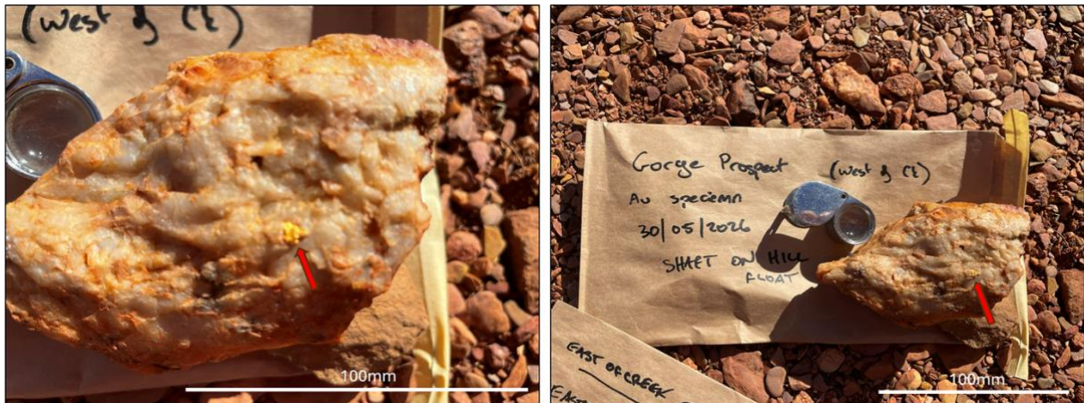
Figure 3 - Visible gold in a quartz vein sample understood to have been sourced from mullock heaps associated with the northern-most western shaft at the Gorge Mine Prospect. Coarse free gold is observed as a bleb within the quartz vein sample.
