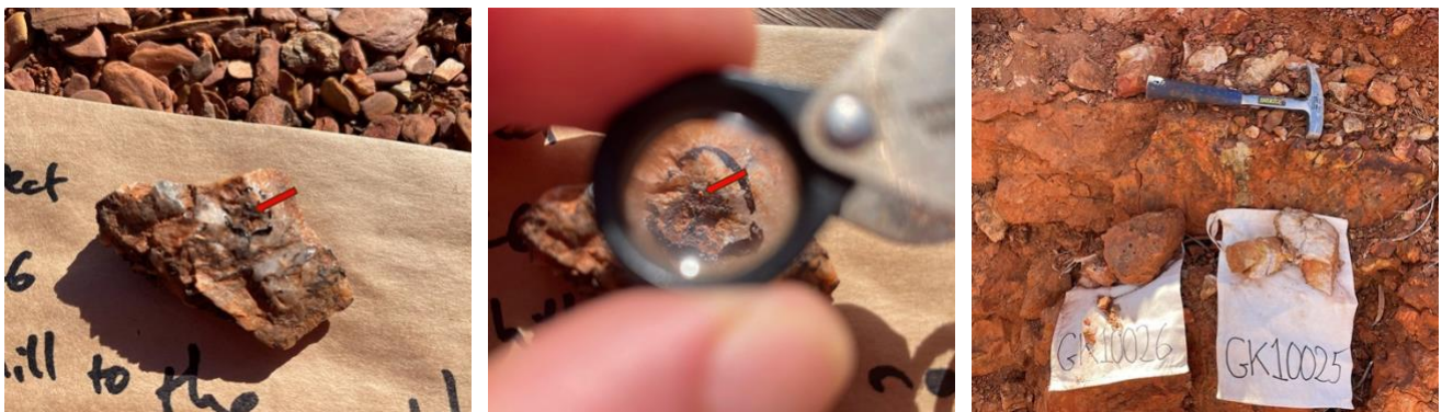
Figure 16 - Rock chip samples collected showing low angle quartz vein with pyrite alteration in wall rock.
