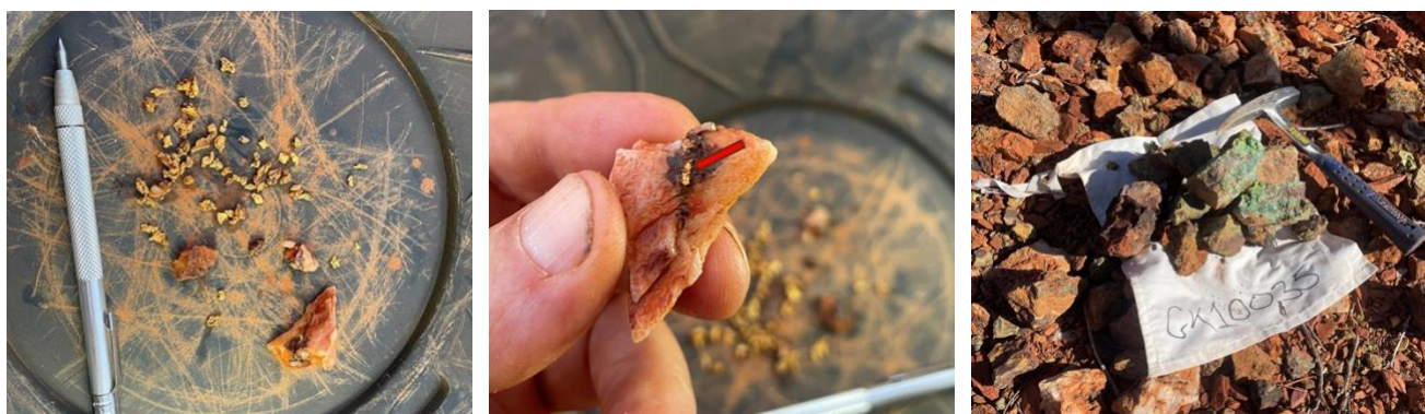
Figure 17 - Gold-bearing material recovered by metal detecting at the Central Zone target area (left), coarse free gold associated with quartz veining and sulphide alteration (middle), and copper-rich gossanous rock samples from the Central Zone Prospect (right).
