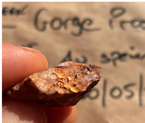
Figure 13 – Visible gold in a quartz vein sample understood to have been sourced from mullock heaps associated with the eastern shaft at the Gorge Mine. Coarse free gold is observed along fractures and veinlets within the quartz vein samples.
