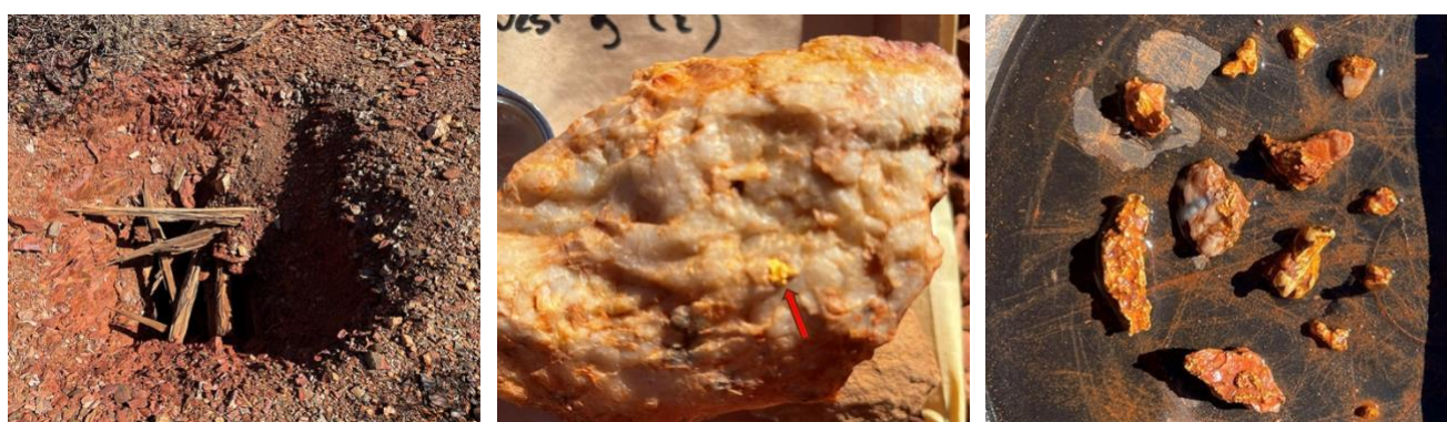
Figure 15 - Historic eastern shaft at the Gorge Mine Prospect (left), visible coarse free gold within quartz vein material (centre), and gold-bearing material recovered during a single day of prospecting on 30 May 2026 (right).
