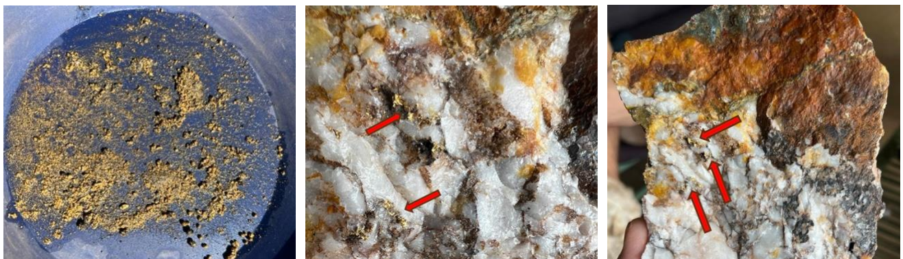
Figure 14 - Historic photographs of quartz vein samples understood to have been sourced from the northern-most western shaft at the Gorge Mine. Pan image shows gold recovered.
